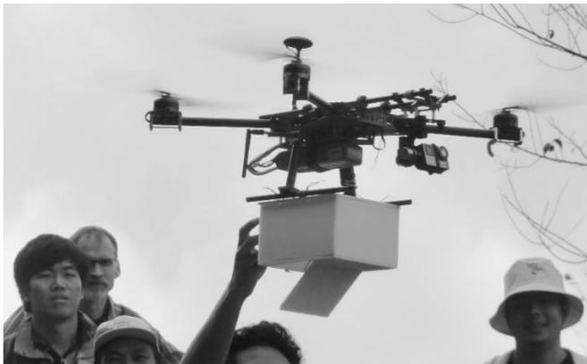
**Figure 1.3 – This drone, demonstrated during the workshop field day, uses a simple box with a trap-door to release seeds into deforested sites.**
