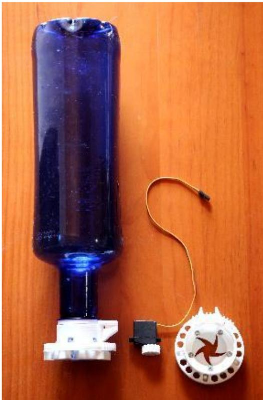
**Figure 7.7 - 3D-printed seed-release system**
