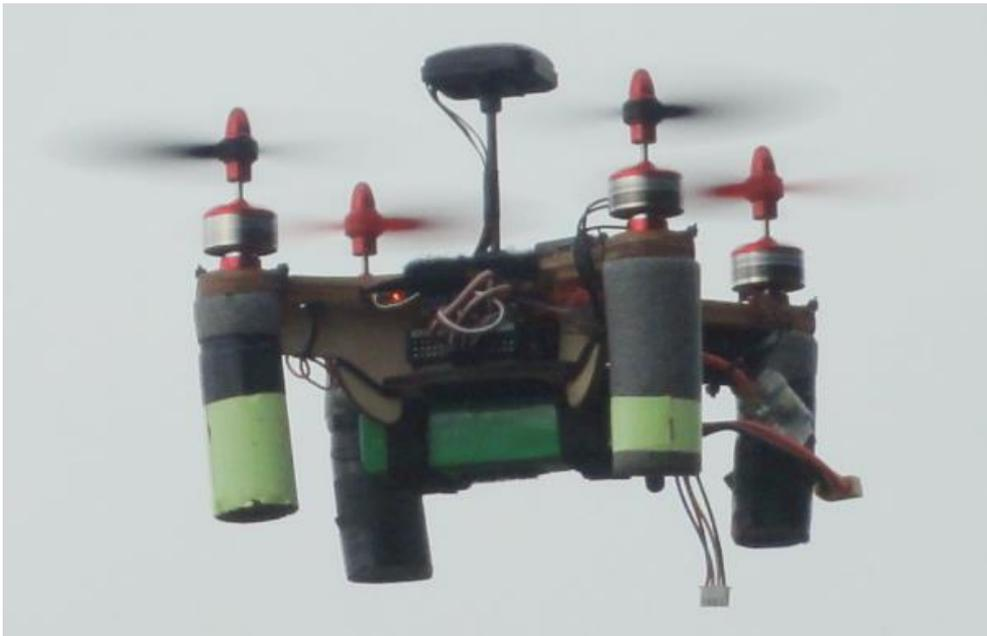
**Figure 7.6 – Controlled by mobile phones with open-source software and constructed from open-source hardware, with biodegradable wooden frames, “flones” are inexpensive and easily repaired. Thus, they are ideal UAVs for citizen-based ecological actions.**
