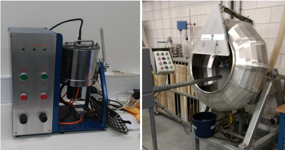
Figure 8.3 – Seed-coating equipment, lab-scale rotary coater on the left, rotating pan on the right.
