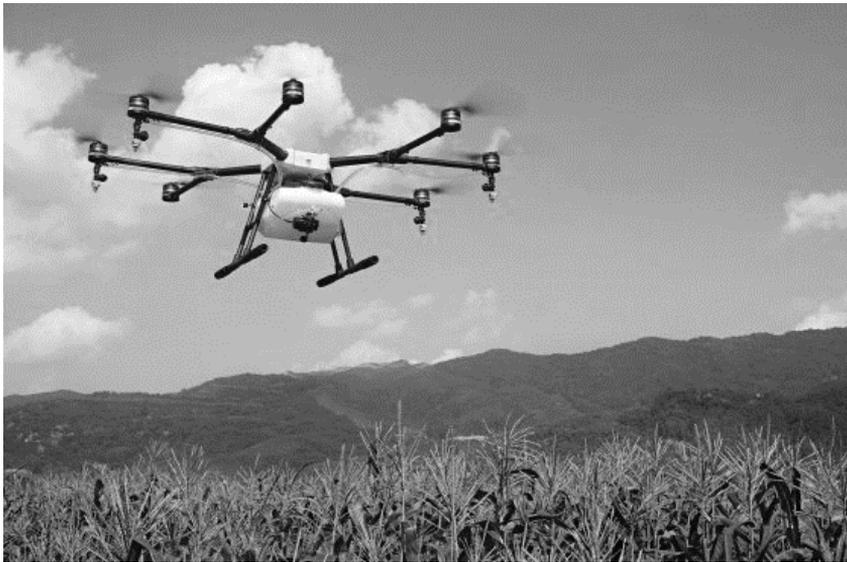
**Figure 9.3 – DJI’s Agras MG-1S is an eight-rotor craft spanning 1.47 m with a 10-litre liquid capacity. It is priced at US\$15,000 (Photo: DJI)**
