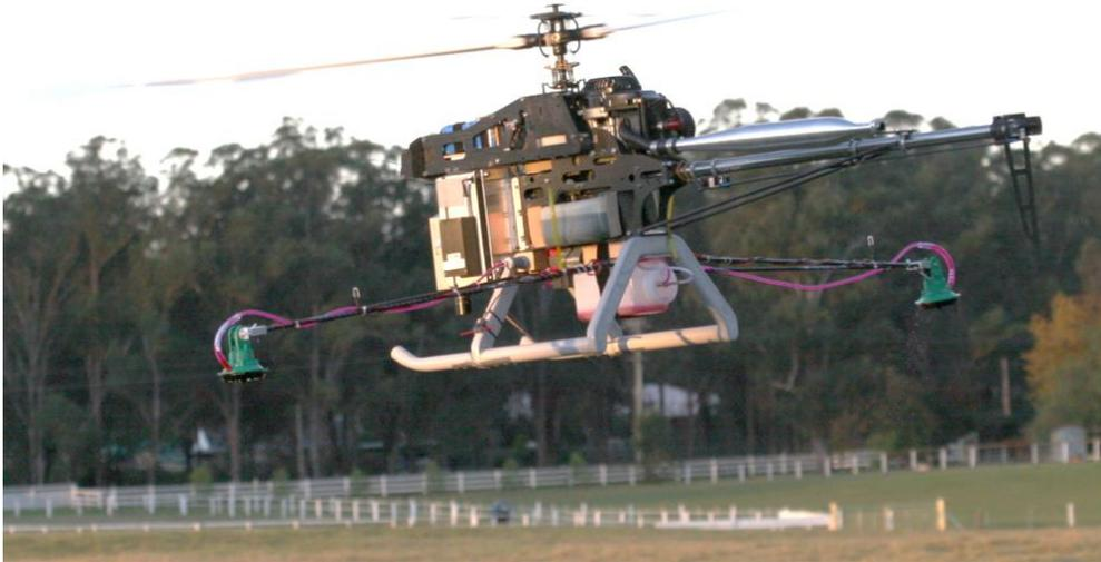
**Figure 9.6 – An auto-piloted mini helicopter, used for weed control**
