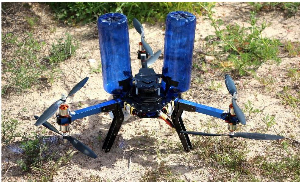
**Figure 7.2 - 3D-Robotics' Y6 hexacopter adapted to carry two seed dispensers**
