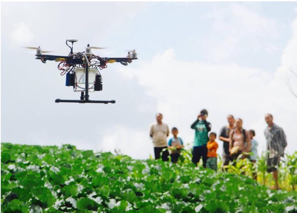
**Figure 10.3 - Testing of auto-spraying for weed management in an agroforestry system**
