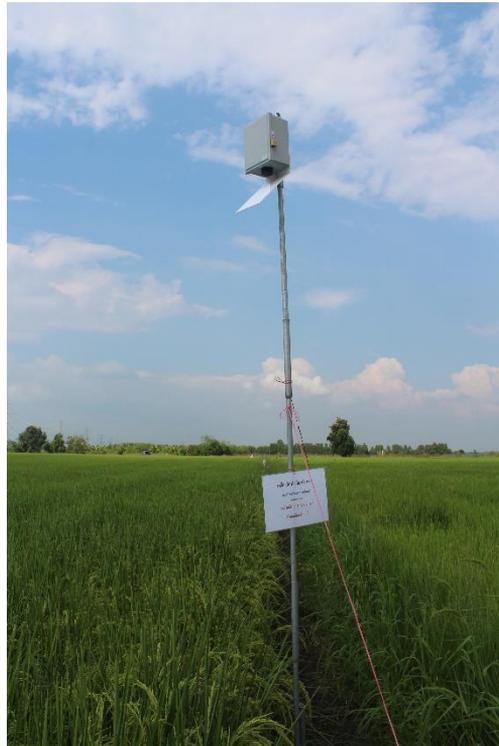
Figure 13.1 A bat acoustic monitoring station; a bat detector is kept in the box
