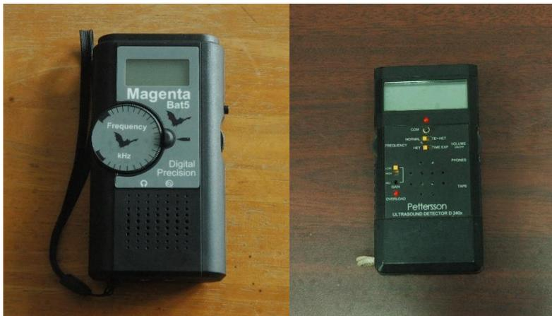
Figure 13.2 A heterodyne bat detector (left) and a time expansion bat detector (right)
